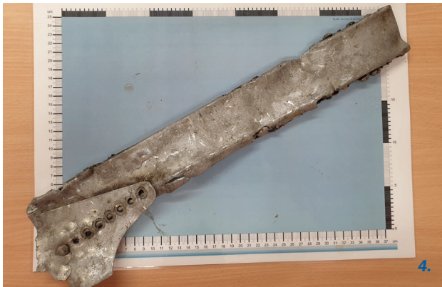
Image 4 , an aircraft component which appears to be a wing rib brace from a B17; Image 5 , an aircraft component with paint still visible; Image 6 , the paint in greater detail, revealing a potential camouflage colour/pattern; Image 7 , an engine valve; and Image 8 , munitions discovered in the same cargo and therefore possibly relating to the same aircraft wreckage.
