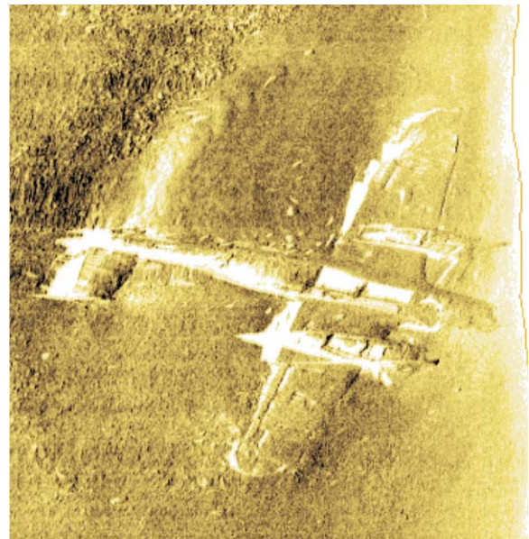
Sidescan sonar image of the possible Luftwaffe Dornier on the seabed off the coast of Kent
